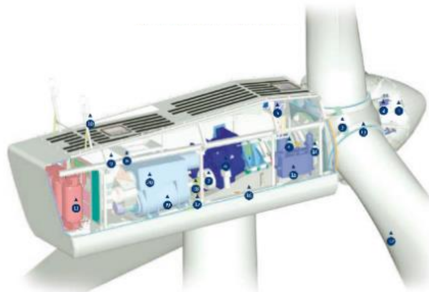
Figure 7.3. Vestas V90-1.8/2.0 MW Components
